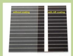
The glare from solar farms could be a thing of the past, thanks to new research. Researchers have developed a multi-layer anti-reflection coating for glass surfaces, which reduces the sun's reflection from photovoltaic panels while at the same time improving their efficiency. It is applied using the same technology as that used for depositing anti-reflection coatings on eye glasses.
