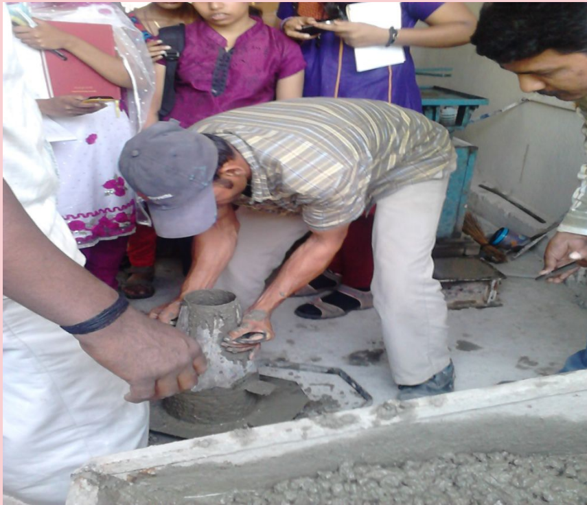
Demonstration of Slump test at AVS Concrete
